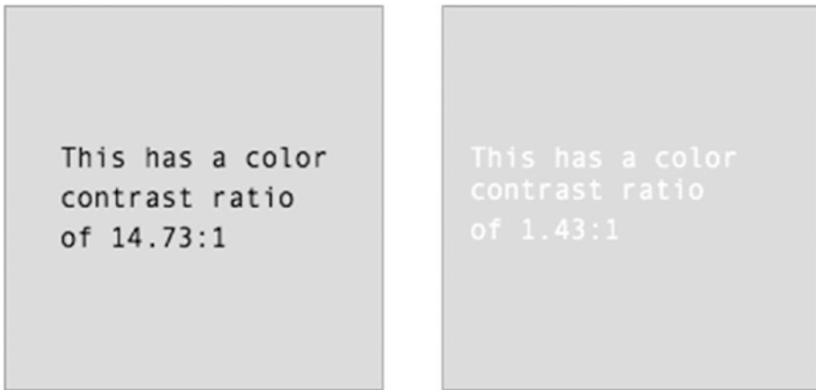
Figure 2-9. Color contrast ratios according to WCAG 2.1. The left image is accessible, while the right image is not
